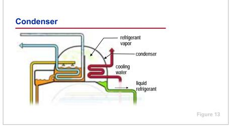
Inside the **condenser**, cooling water flows through tubes and the hot refrigerant vapor fills the surrounding space. As heat transfers from the refrigerant vapor to the water, refrigerant condenses on the tube surfaces. The condensed liquid refrigerant collects in the bottom of the condenser before traveling to the expansion device.
